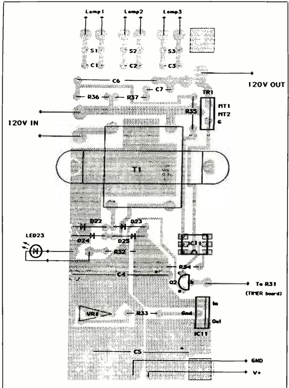
Fig. 7. Wiring guide for power-supply/controller board.
